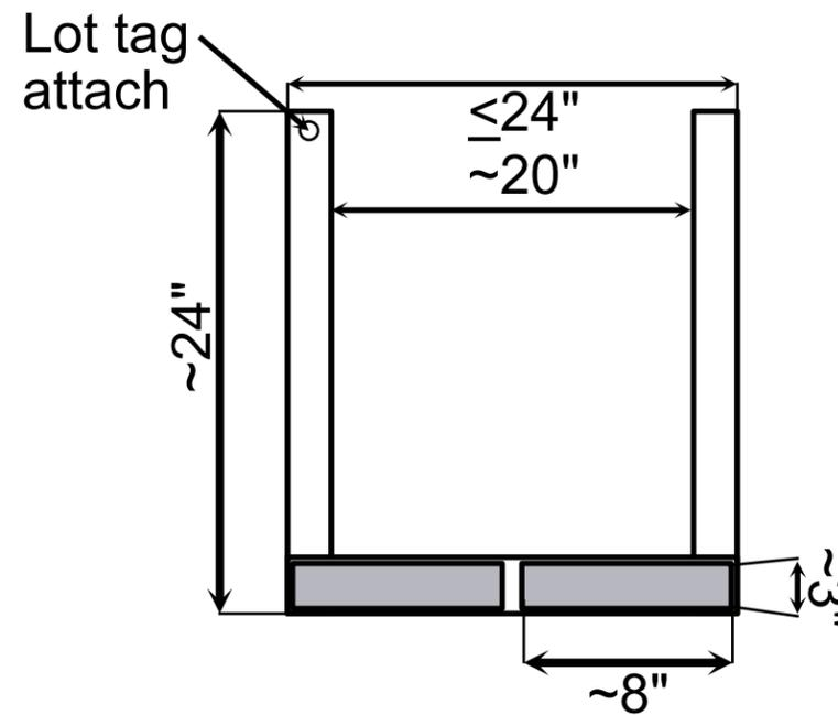
8" x 3" channel for illustration, fabricator should size to fork tine sizes in use
