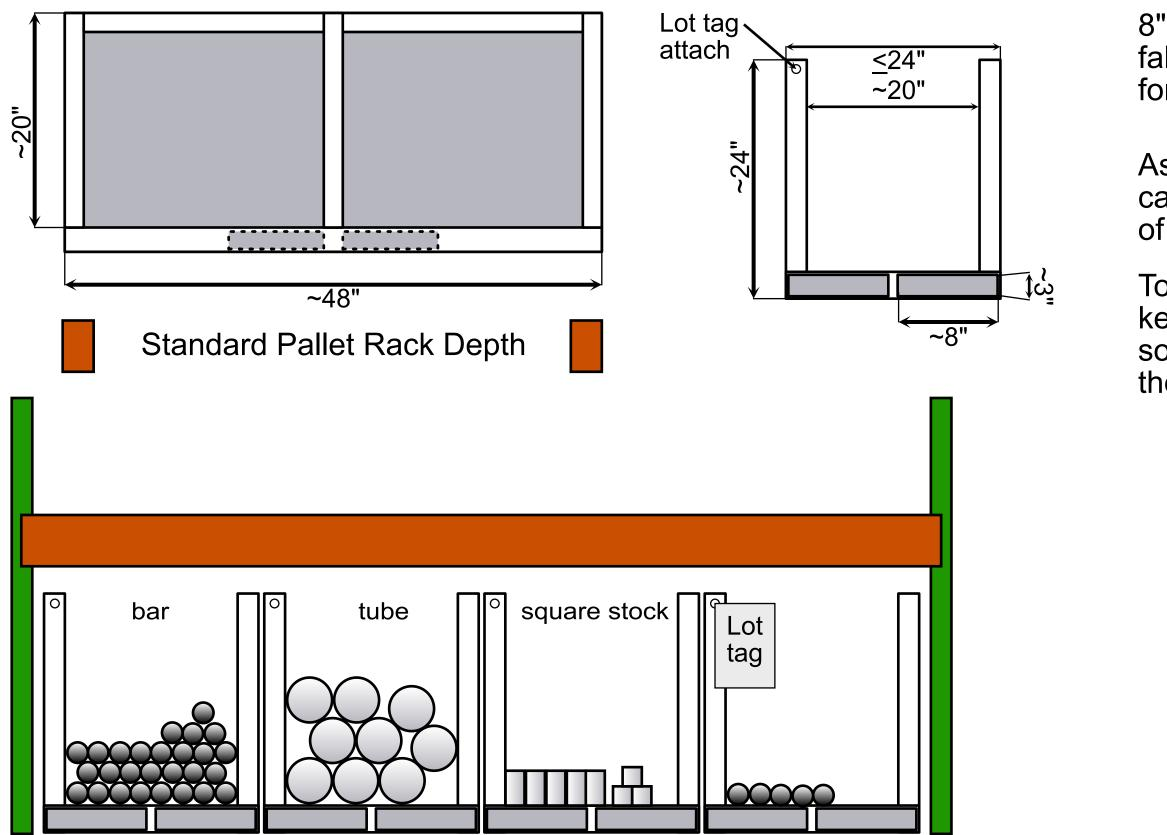
High density for materials, round bar, tube, etc. Designed to be 4x per pallet rack shelf
